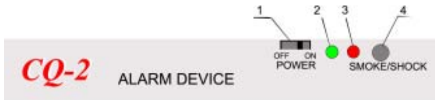
Fig.1 CQ-2 Alarm Device Switch Panel
