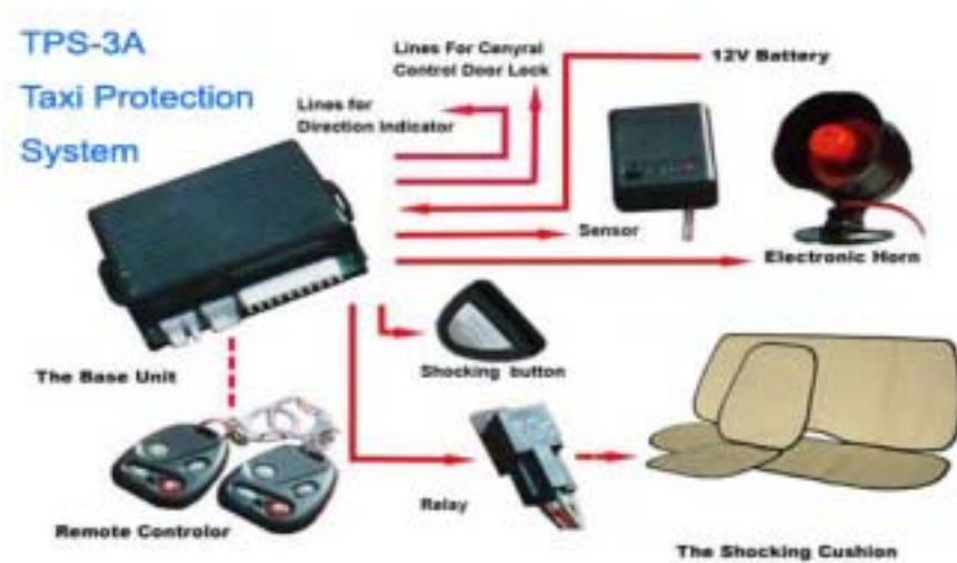
Fig8 TPS-3A Taxi Protection System
