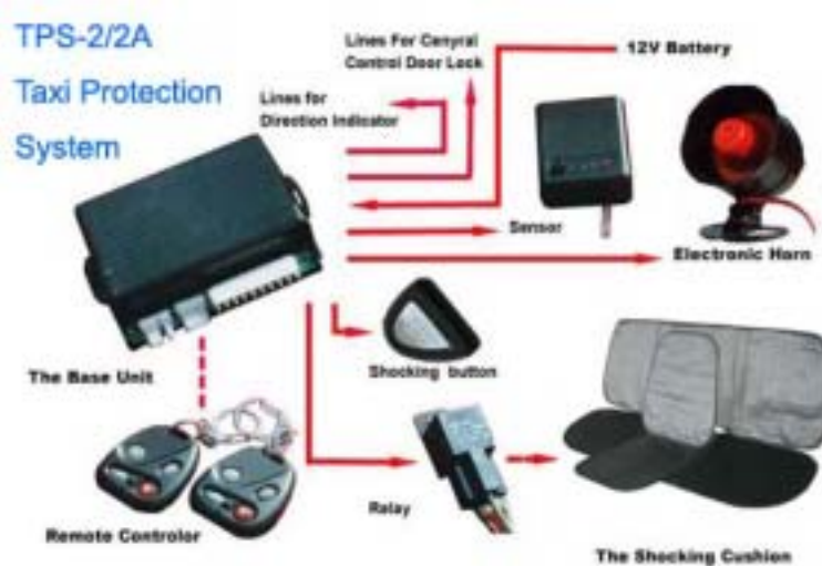
Fig7 TPS-2/2A Taxi Protection System
